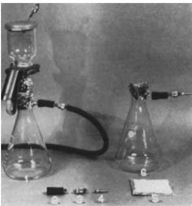
Fig. 1.—Assembled filtration unit. Key: 1, Pyrex suction flask for filtration; 2, female adapter; 3, Swinny adapter with air filter; 4, male adapter; 5, gauze square; 6, Pyrex suction flask for incubation.
